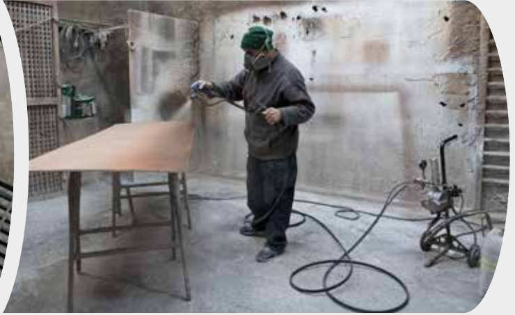
Wood varnish spraying.
