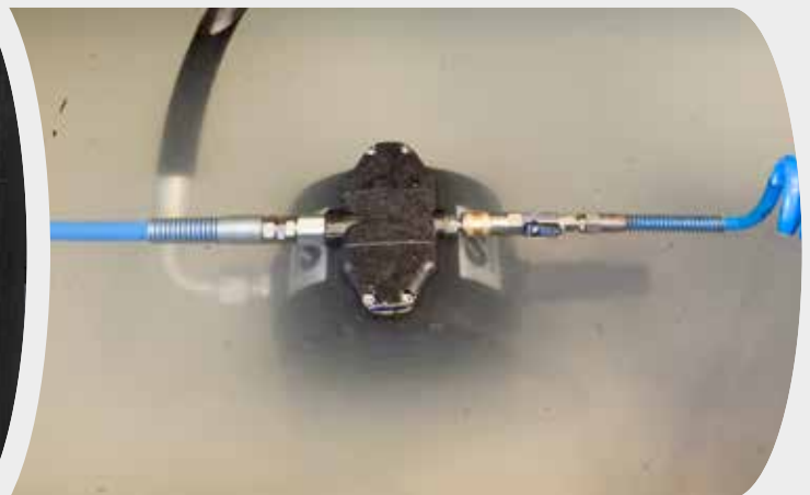
Submersed pump application.
